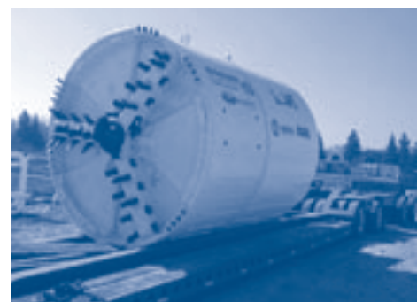
The UNWI 1 & 2 tunnel will be constructed using a similar tunnel boring machine.
